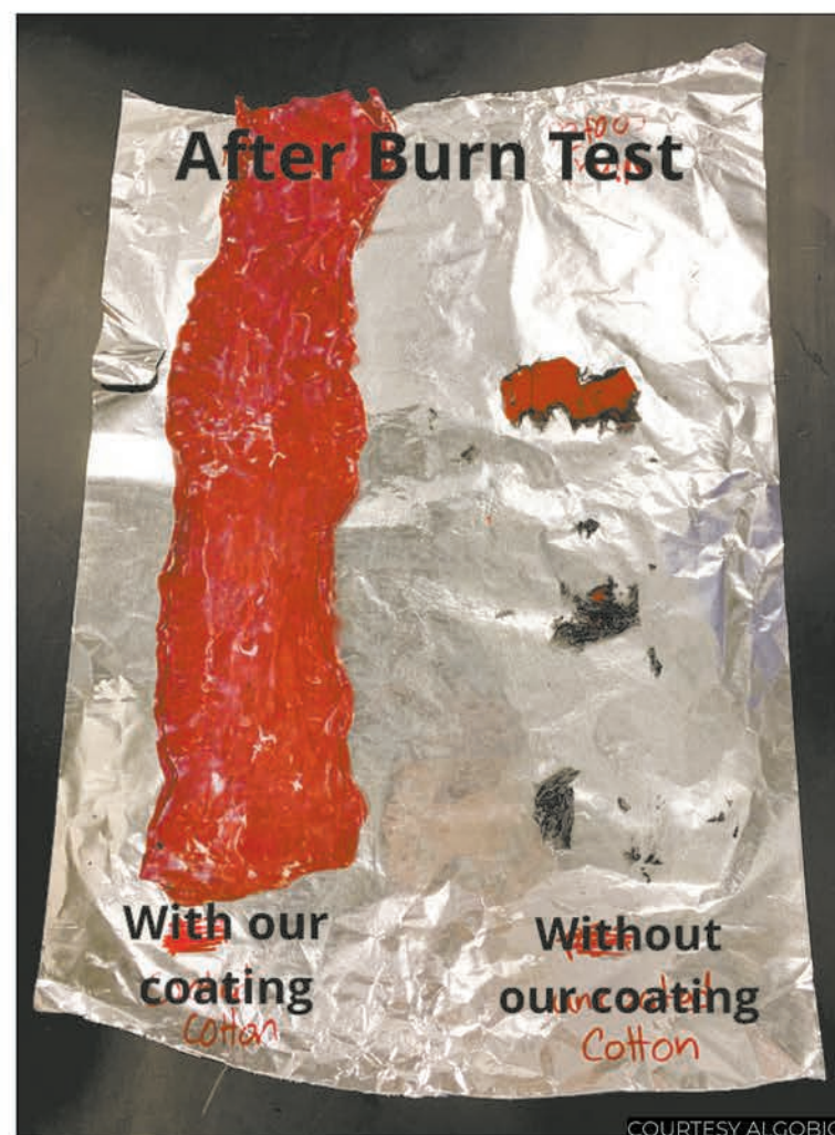
Burn test of AlgoBio flame retardant on cotton
